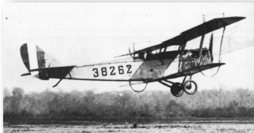
The Curtiss JN4-H biplane depicted in the stamp vignette, flew the mail on the first US airmail route.
